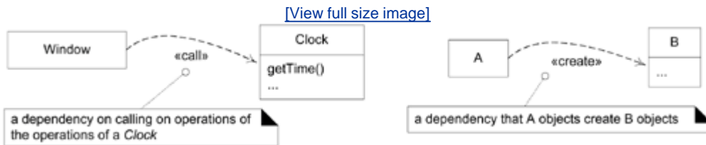
Figure 16.11. Optional dependency labels in the UML.
