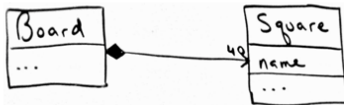
Figure 17.5. In a DCD of the Design Model, Board has a composite aggregation association with Squares . We are applying Creator in a static model.
