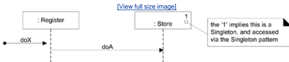
Figure 15.6. Singletons in interaction diagrams.
