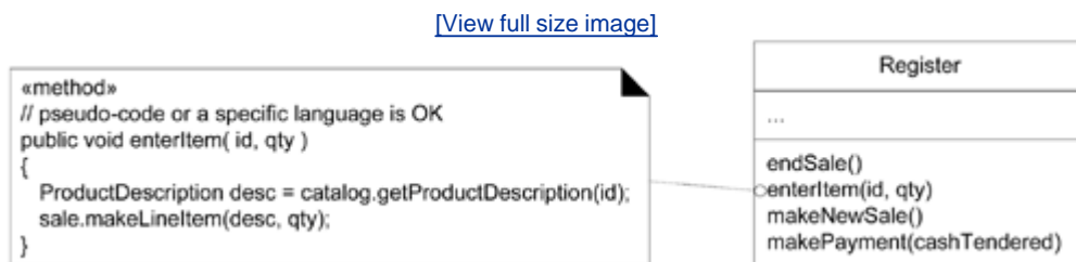
Figure 16.7. How to show a method body in a class diagram.
