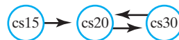
FIGURE 28-13 An impossible prerequisite structure for three courses, as a directed graph with a cycle
