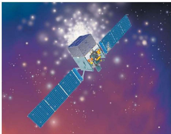
▲ FIGURE 5.35 Gamma-Ray Astronomy (a) The Fermi Gamma-Ray Space Telescope , shown here in an artist's conception, was named after Enrico Fermi, an Italian-American scientist who did pioneering work in high-energy physics. The wide arrays are solar panels to power the spacecraft; the box amidship contains layers of tungsten that detect the gamma rays. (b) A typical false-color gamma-ray image—this one showing the remains of a violent event (a supernova) in a region named W44. The gamma rays are shown mainly in magenta. (NASA)
