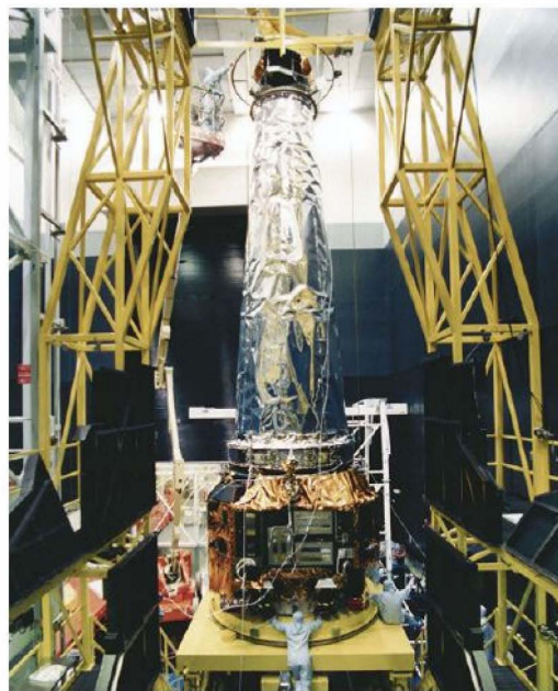
▲ FIGURE 5.33 Chandra Observatory The Chandra X-ray telescope is shown here during the final stages of its construction in 1998. The left end of the mirror arrangement, depicted in Figure 5.32, is at the bottom of the satellite as oriented here. Chandra's effective angular resolution is 1'' , allowing this spacecraft to produce images of quality comparable to that of optical photographs. Chandra now occupies an elliptical orbit high above Earth; its farthest point from our planet, 140,000 km out, reaches almost one-third of the way to the Moon. Such an orbit takes Chandra above most of the interfering radiation belts girdling Earth (see Section 7.5) and allows more efficient observations of the cosmos. (NASA)
