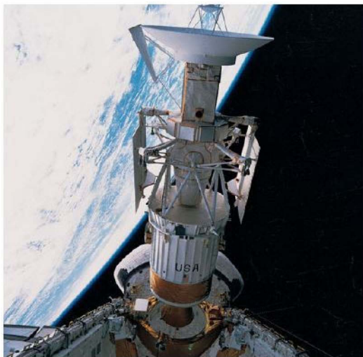
▲ FIGURE 6.10 Magellan Orbiter The U.S. Magellan spacecraft was launched from the space shuttle Atlantis (at bottom) in May 1989 on a mission to explore the planet Venus. The large radio antenna at the top was used both for mapping the surface of Venus and for communicating with Earth. Contrast the relatively delicate structure of this craft, designed to operate in space, with the much more bulky design of the Venus lander shown in Figure 6.9. (NASA)
