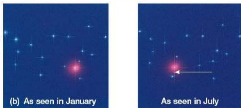
Interactive FIGURE 17.1 Stellar Parallax (a) For observations of stars made 6 months apart, the baseline is twice the Earth–Sun distance, or 2 AU. Compare with Figure 1.30, which shows the same geometry, but on a much smaller scale. (b) The parallactic shift (exaggerated here, and indicated by the white arrow in this drawing) is usually measured photographically, as illustrated by the red star seen here. Images of the same region of the sky made at different times of the year are used to determine a star's apparent movement relative to background stars. This basic measurement is key to understanding the properties of stars throughout the universe.
